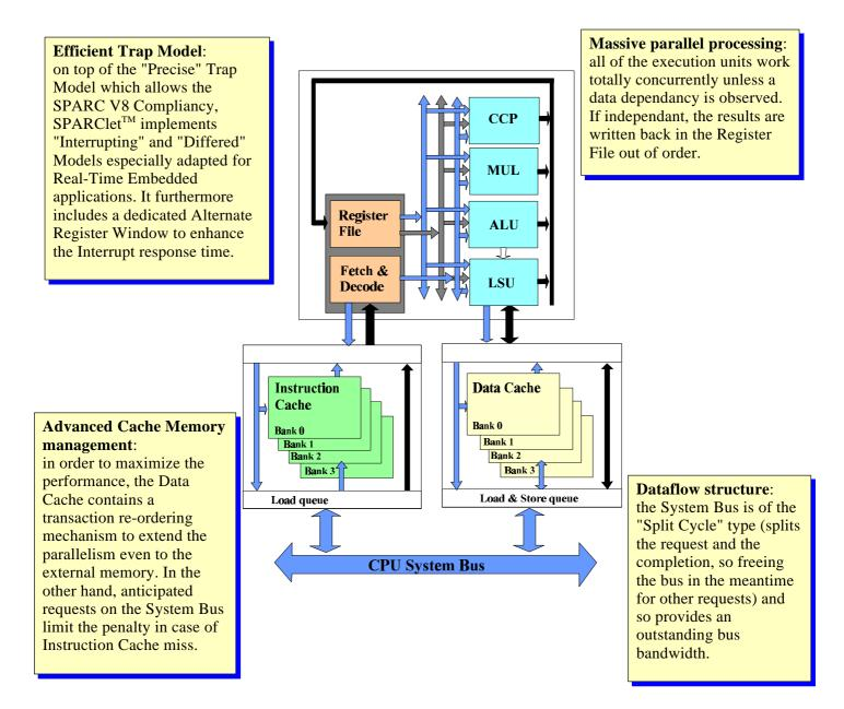
The SPARC V8 Instruction Set has been enriched with new instructions: SCAN (bit scanning), Shuffle (bit/nibble/byte/half-word swapping), and the instructions dedicated to the on-chip coprocessors (MUL and CCP for the TSC701).
